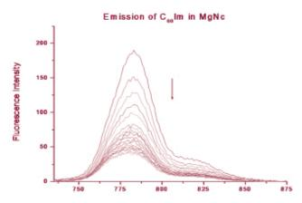
Figure 7. Fluorescence intensities of MgNc upon the increasing addition of C<sub>60</sub>Im in o-dichlorobenzene.
