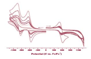
Figure 8. Cyclic voltammogram of the MgPc upon increasing addition of C<sub>60</sub>Im (0.2, 0.6, 0.8, I.O, I.5 and 2.0 eq.) in o-dichlorobenzene, 0.1 M (TBA)  $ClO_4$ . Scan rate = 100 mV/s.
