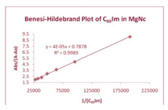
Figure 5. Benesi-Hildebrand plot of magnesium tetra-tert-butylnalphthalocyanine coordinated with C<sub>60</sub>Im. The binding constant was determined to be  $1.96 * 10^4 \,\mathrm{M}^{-1}$ .
