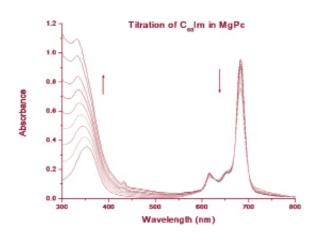
**Figure 2.** Ultraviolet/Visible spectra during the titration of MgPc on the addition of C<sub>60</sub>Im in o-dichlorobenzene, a noncoordinating solvent.
