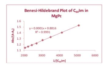
Figure 4. Benesi-Hildebrand plot of magnesium tetra-tert-butylphthalocyanine coordinated with C<sub>60</sub>Im. The binding constant was determined to be 8.82 \*10<sup>3</sup> M<sup>-1</sup>.
