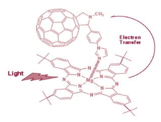
Scheme I. Magnesium phthalocyanine - fullerene donor-acceptor dyad. The arrows show the occurrence of photoinduced electron transfer.
