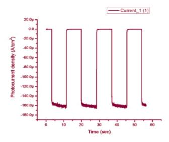
Figure 10. Current switching (I-t) of a FTO/ TiO /MgPc electrode under AMI.5 condition.
