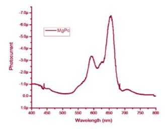
Figure II. The photocurrent action spectrum FTO/TiO<sub>3</sub>/MgPc.
