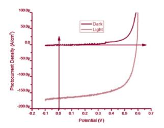
Figure 12. The I-V characteristics of TiO /ITO/ MgPc.
