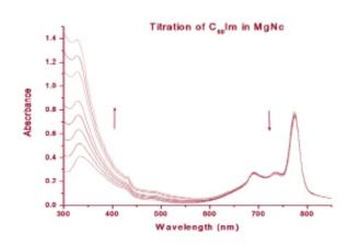
**Figure 3.** Ultraviolet/Visible spectra during the titration of MgNc on the addition of  $C_{60}$ Im in o-dichlorobenzene, a noncoordinating solvent.
