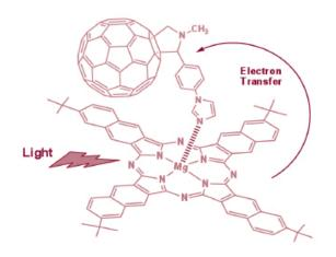
Scheme 2. Magnesium naphthalocyanine - fullerene donor-acceptor dyad. The arrows show the occurrence of photoinduced electron transfer.
