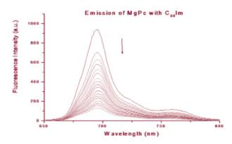
**Figure 6.** Fluorescence intensities of MgPc in the increasing addition of C<sub>60</sub>Im in o-dichlorobenzene.
