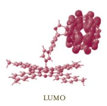
Figure 9. DFT/B3LYP(\*) optimized structure of MgPc. HOMO is located on MgPc and LUMO located on fullerene.
