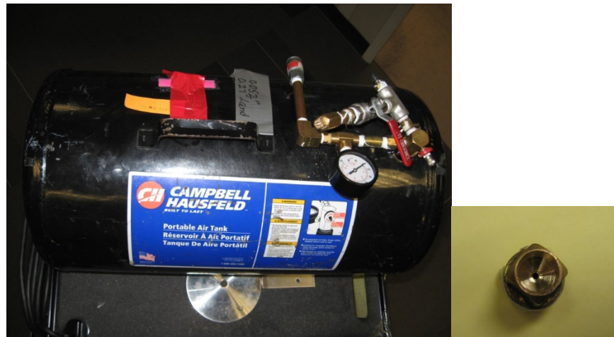
Figure 2. Photograph of the Air Tank and Respective Attachments for Venting Data Collection
