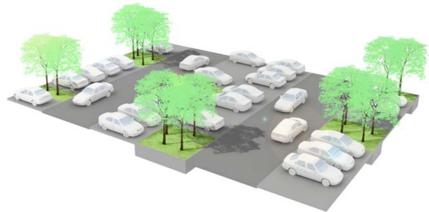
Proposed Parking Lots Incorporate Tree Plantings for Shade and Stormwater Management
