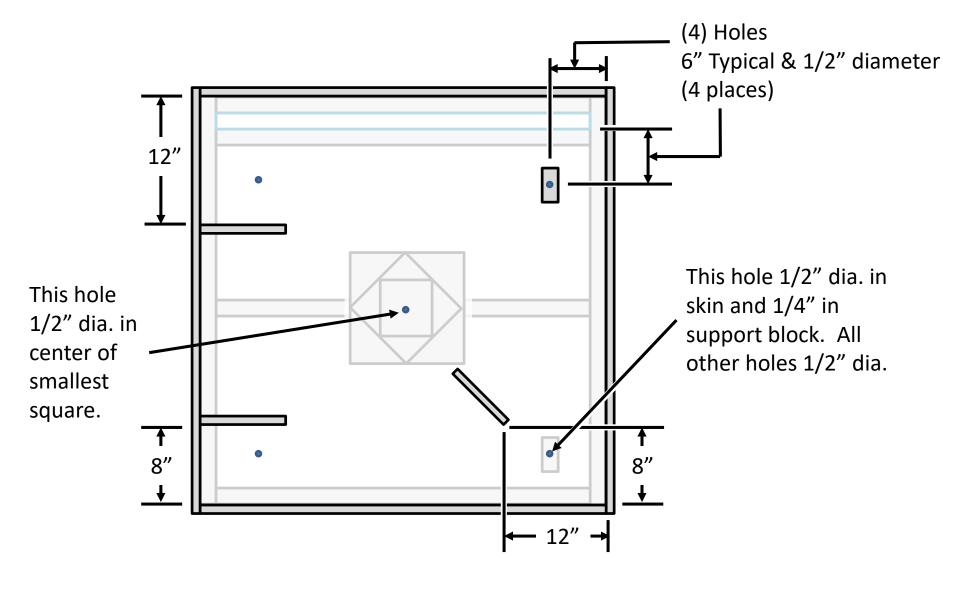
Addition of (3) 1.5" x 8" walls, raised block, (4) 1/2" holes, (1) support block beneath plywood, and (1) 1/4" hole as shown.
