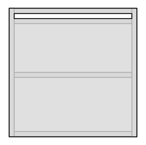
Apply 48" x 48" Luan plywood removing the 45" x 1.5" narrow strip as shown here.
