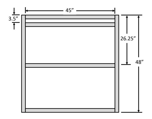
Assemble 2" x 2" components in the configuration shown above.
