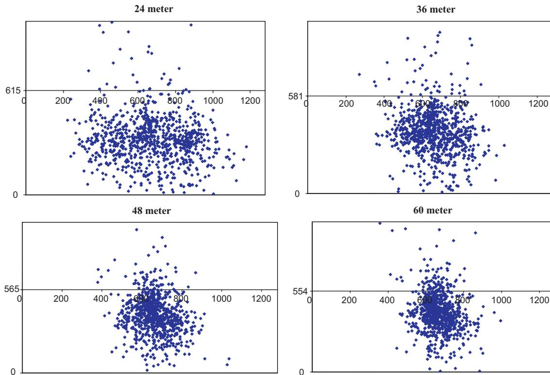
**Fig. 7.** Location of eye fixations immediately prior to a light change. The fixations are for all subjects for each light change and are presented in screen units (pixel position). Separate graphs are presented for each distance that a light change occurred.
