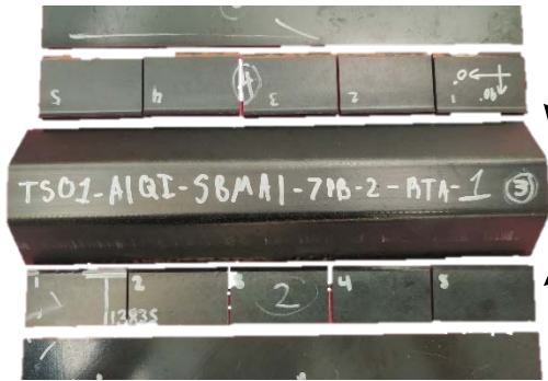
Traveler Coupons from bonded flange region to evaluate saturation rate during environmental conditioning Traveler mass ≈ 10 g
