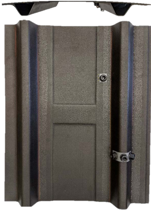
2-Stringer panel with added mass (2cm diameter steel nuts) simulating damage
