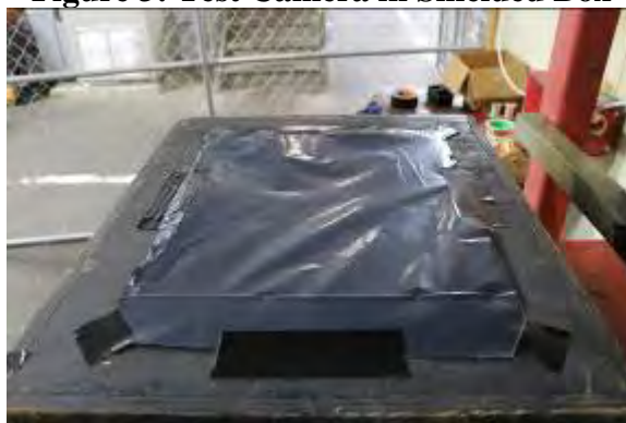
Figure 4: Blowout Film for Pressure Changes in Test Chamber
