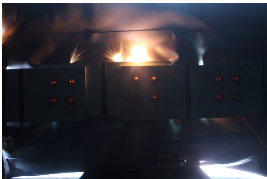
Figure 76: CF7-4C20A-4-Tail Side-Test Photo-Shot 1-20 kA
