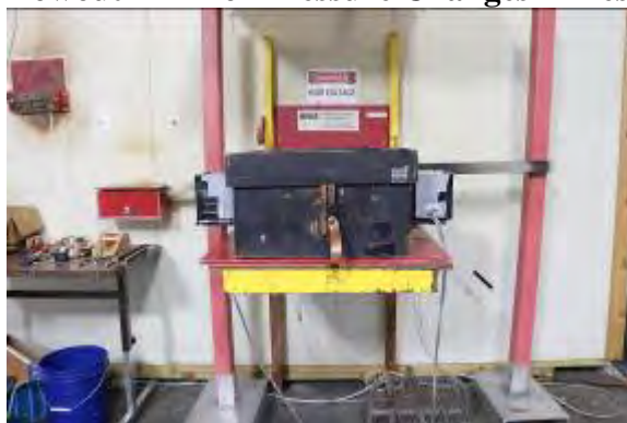
Figure 5: DEL Generator Test Setup – Test Chamber with Cameras in Shielded Boxes
