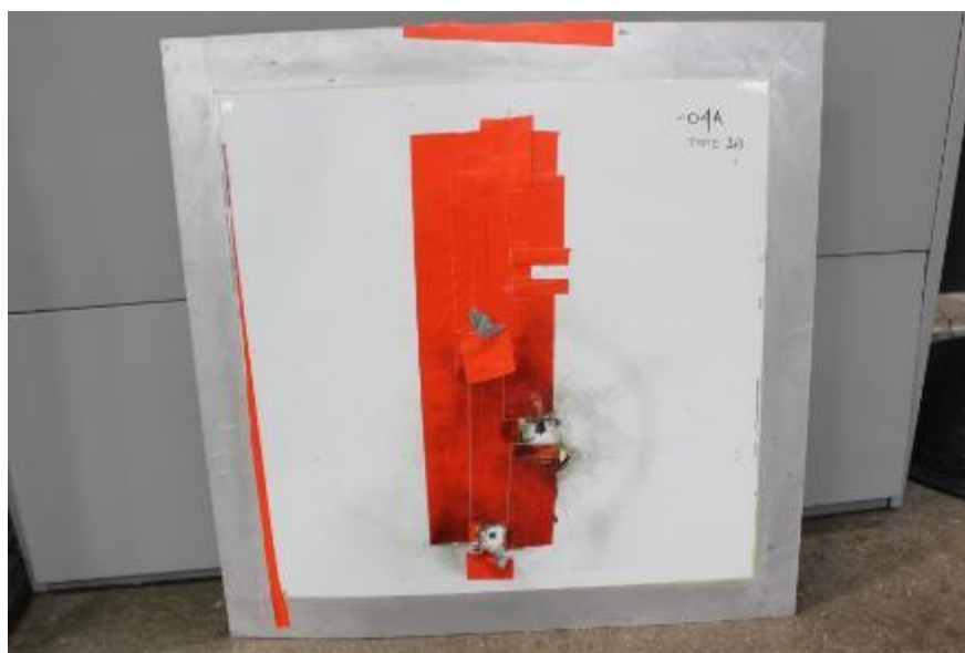
Figure B-20: Arc Entry Test -04A-Post-Test-Front
