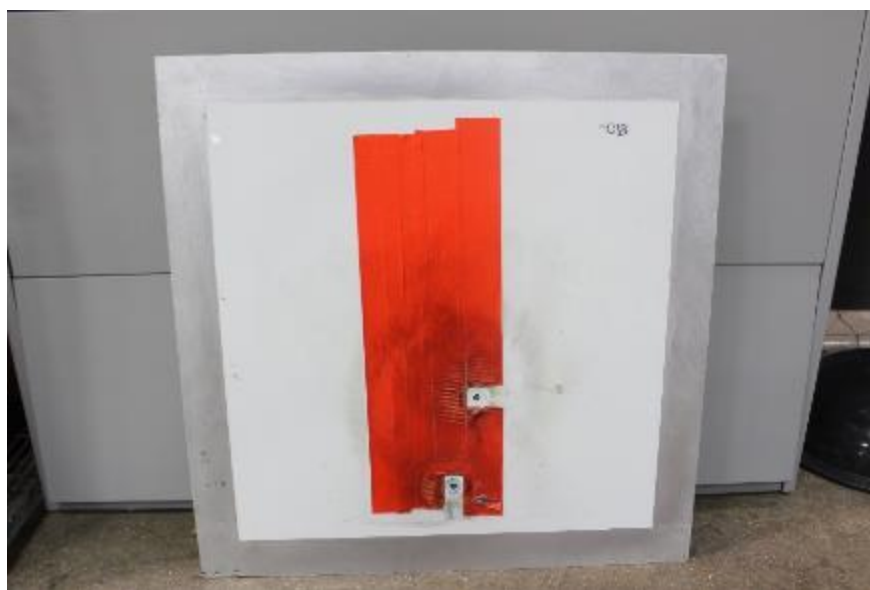
Figure B-8: Arc Entry Test -01B-Post-Test-Front
