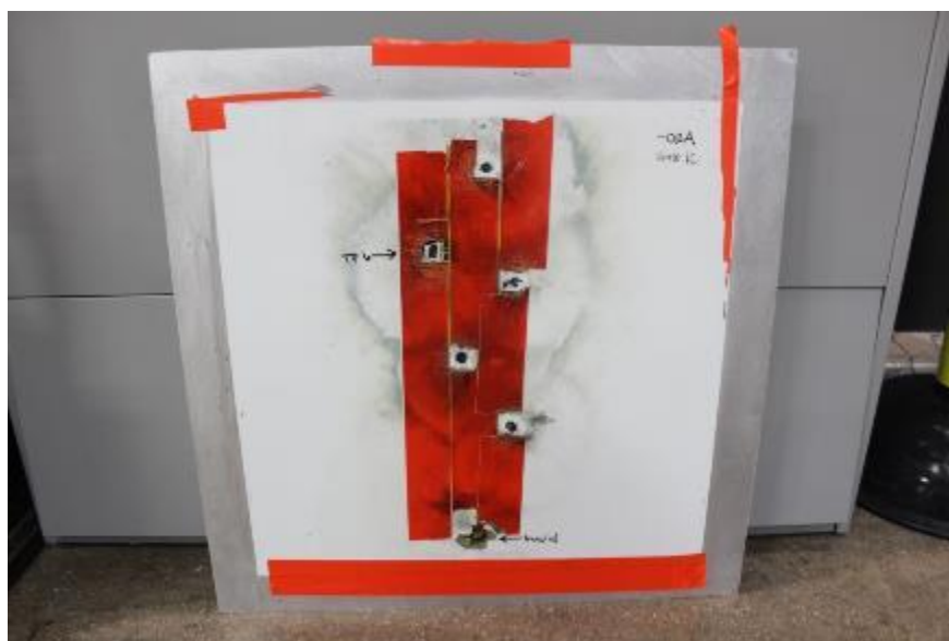
Figure B-12: Arc Entry Test -02A-Post-Test-Front
