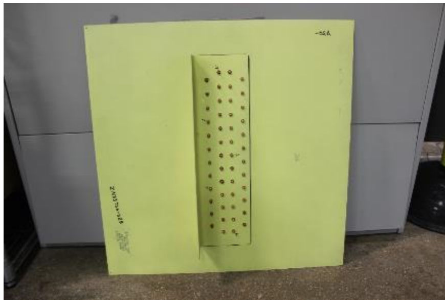
Figure B-11: Arc Entry Test -02A-Post-Test-Back
