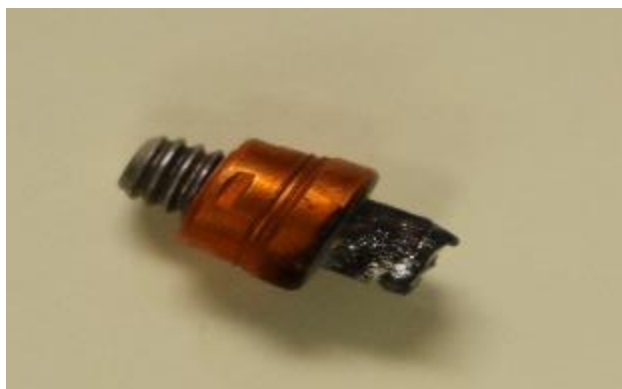
Figure 9: Fastener after being expelled from panel (Panel -04A TP1)
