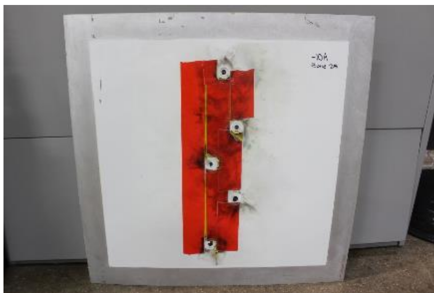
Figure B-48: Arc Entry Test -10A-Post-Test-Front
