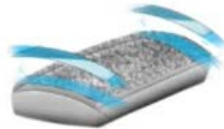
Lay-up Conexus-layer in joining areas
