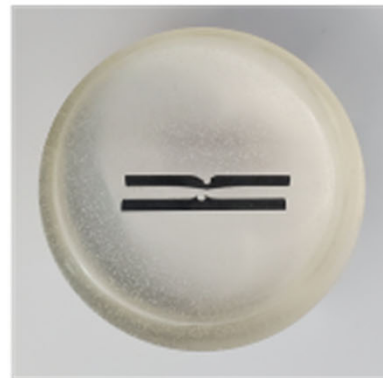
Potted specimen in clear epoxy
