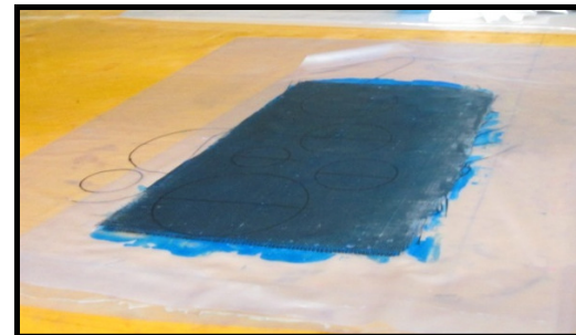
Element scarf sanded in preparation for repair
