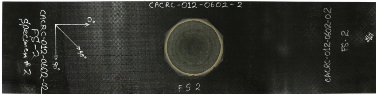
CACRC-012-0602-2 Repaired Element (CACRC Prepreg Repair)
