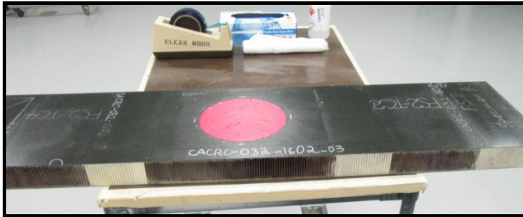
Adhesive application – prepreg repair
