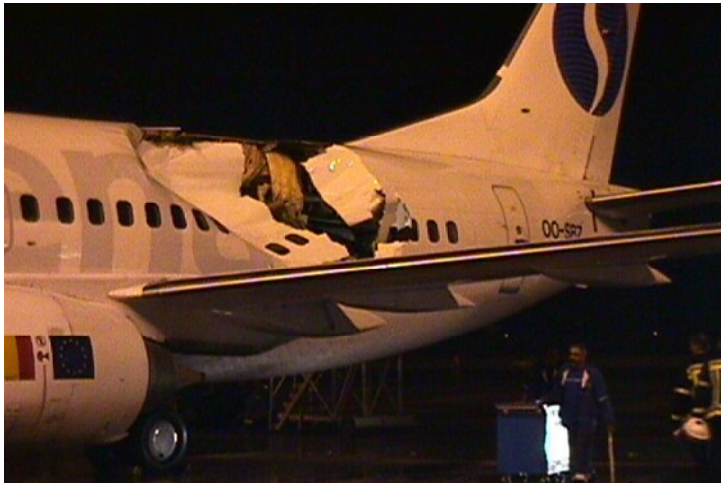
In-Service Damage, Courtesy Eric Chesmar, UAL [1]
