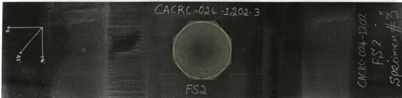
CACRC-024-1202-3 Repaired Element (CACRC Prepreg Repair)
