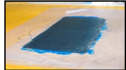
Wet lay-up resin impregnation
