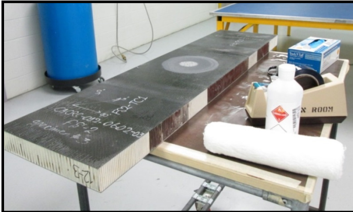
Element scarf sanded in preparation for repair
