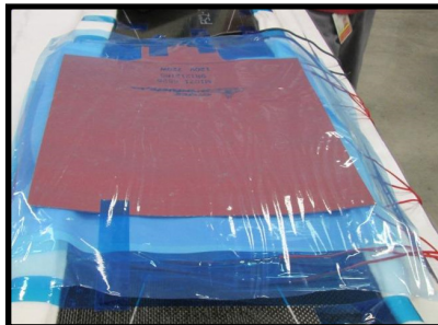
Heat Blanket Application
