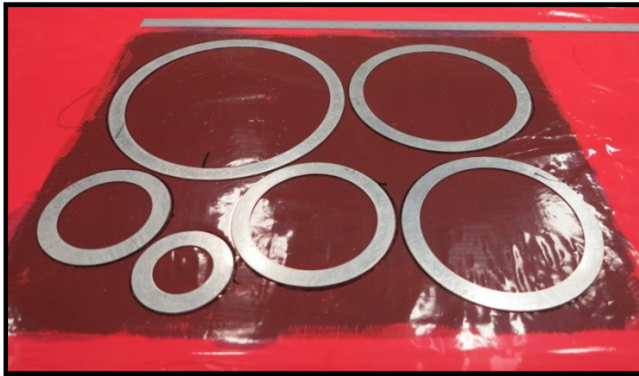
Wet lay-up ply impregnation
