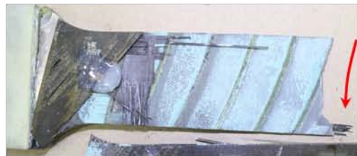
(b) Failure surface –OML side
