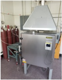
Nabertherm LH 120/12 w/ P470 controller and gassing box (Argon treatment)
