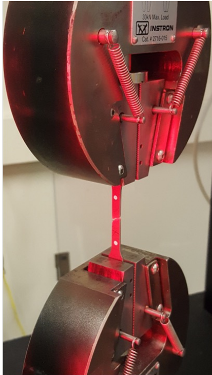
ASTM E8, Subsize Coupons Clip-on extensometer
