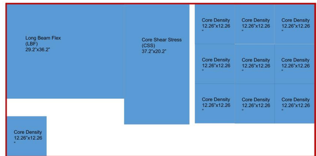
Batch A Sheet 5 0.5" 0.5" border around all panel edges (red) 0.13" added on all sides of all specimens All measurements 0"(W)x90"(L)
