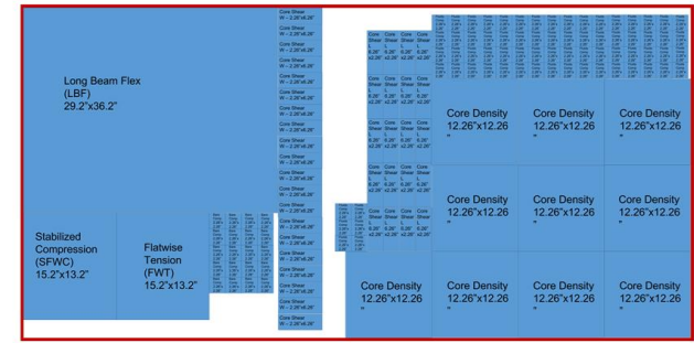
Batch A Sheet 1 0.5" 0.5" border around all panel edges (red) 0.13" added on all sides of all specimens All measurements 0"(W)x90"(L)
