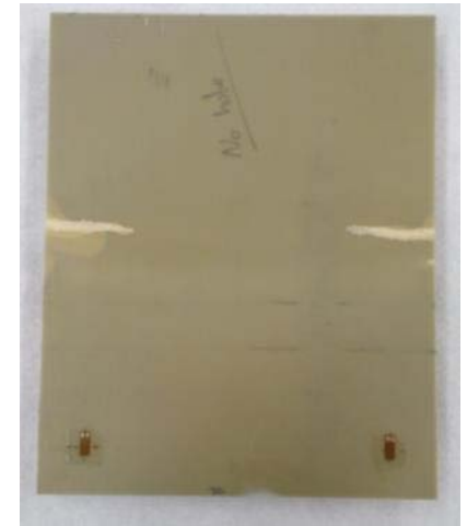
Failure of specimen with no damage
