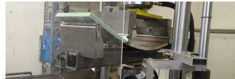
Large deflection using filled core specimen
