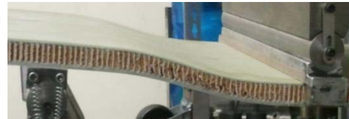
Undesired core shear failure
