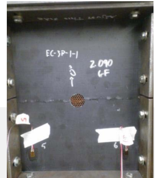
Failure of specimen with 1 in. hole
