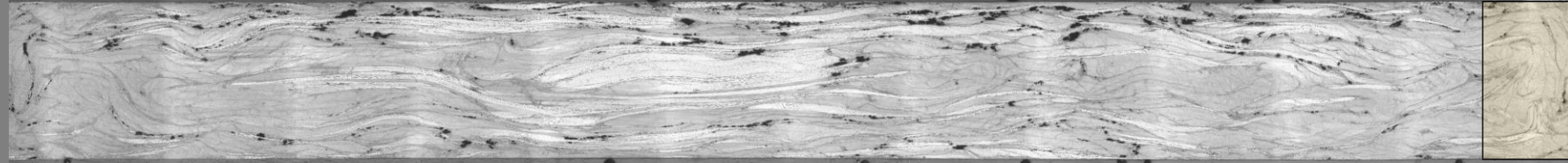
Square Platelet – High Flow 13.5” x 1.5” Panel – 4-7-2 (Transverse 90-degree)
