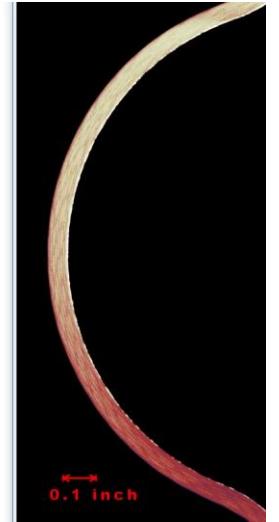
AS4 PW/8552; [90^{\circ}/0^{\circ}]_{2S}
