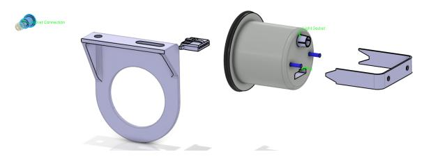
**Select the** *Light Socket* **text on the gauge.** The light socket is assembled to the gauge. A revolute engineering connection is created, meaning it has two degrees of freedom: one linear and one rotational.
