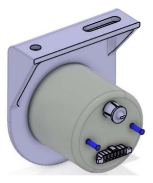
Switch to the Assembly Design workbench and create the necessary engineering connections to assemble the support to the gauge. You will want to add a fix engineering connection constraint to the gauge mount first.
