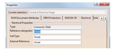
Notice this is defined as a *Connector Shell* (a *Shell*) device. Shells allow single insert connectors to connect via a cavity and a cavity connection point.
