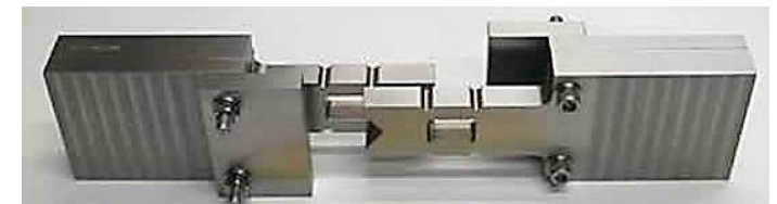
Open hole compression fixture for monolithic composites
