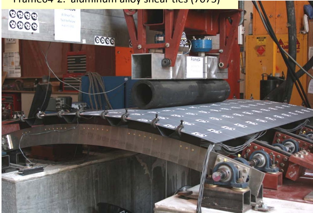
Frame04-2 – Aluminum Alloy (7075) Shear Ties
