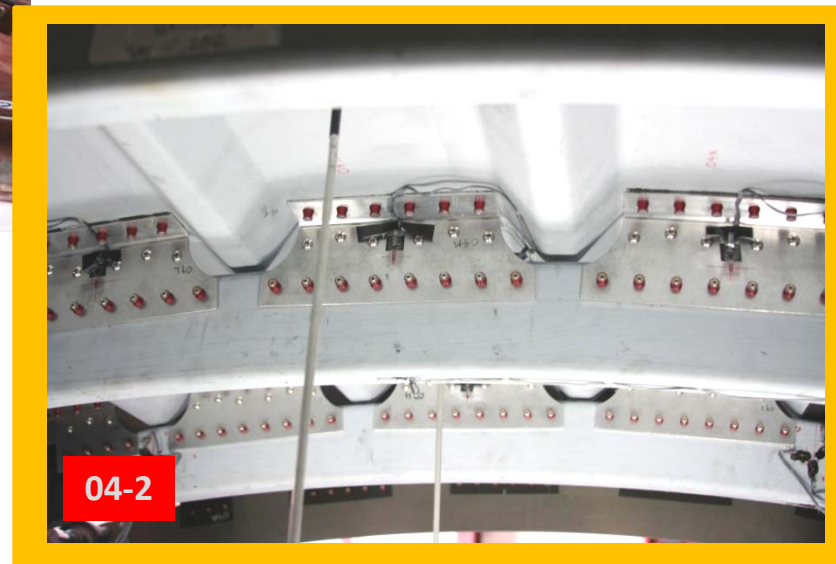
Frame04-2 – Aluminum Alloy (7075) Shear Ties
