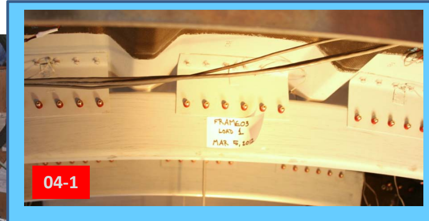
Frame04-1 – Composite Shear Ties
