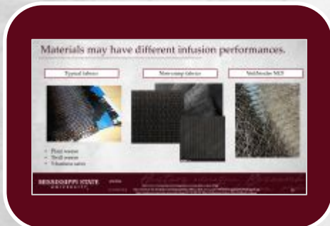
A successful infusion with a specific material set does not all material sets will be successful.
