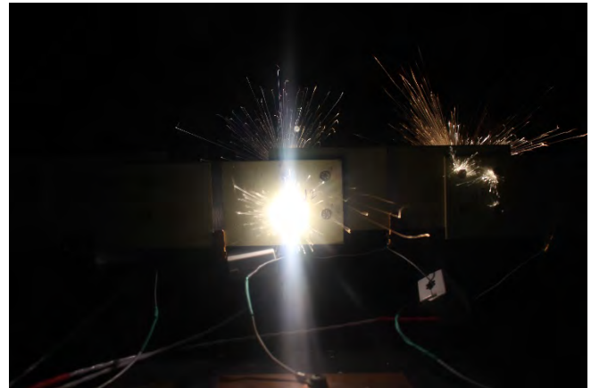
Figure 142: MF3-4T12-2, 10kA, J2 & J3, during test, front
