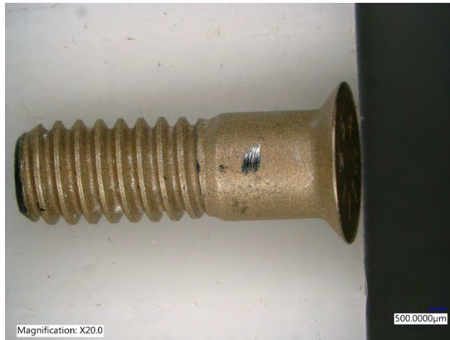
Figure 57: HI KOTE 1 coated fastener
