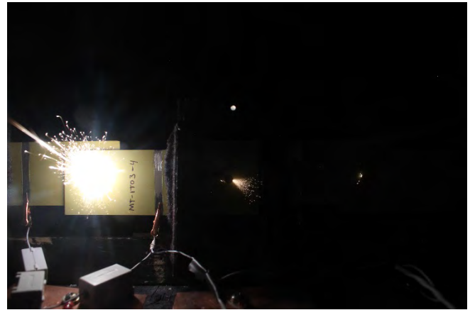
Figure 20: MN-1To3-4, during test, external sparks on all 3 joints
