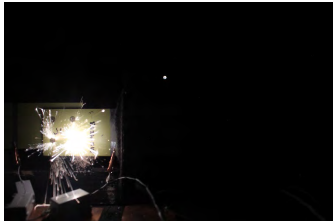
Figure 74: MN-4IO3-3, during test, external spark on J1
