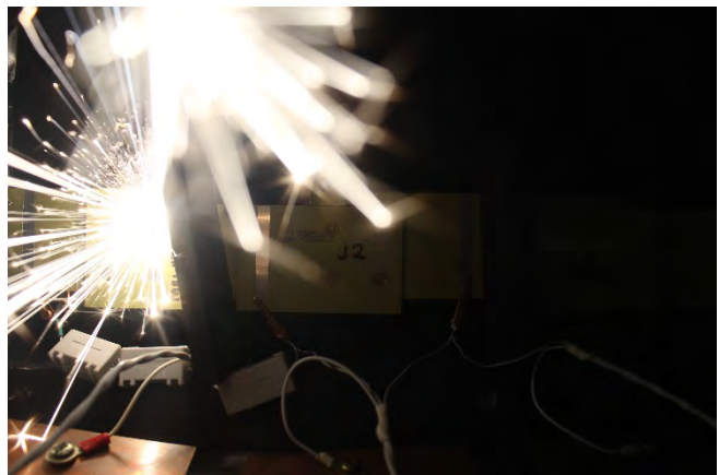
Figure 104: MF1-4T12-2, 0.5kA, J1, during test, front
