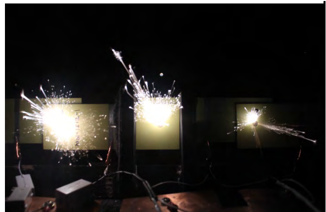
Figure 6: MN-1I12-1, during test, external sparks on all 3 joints
