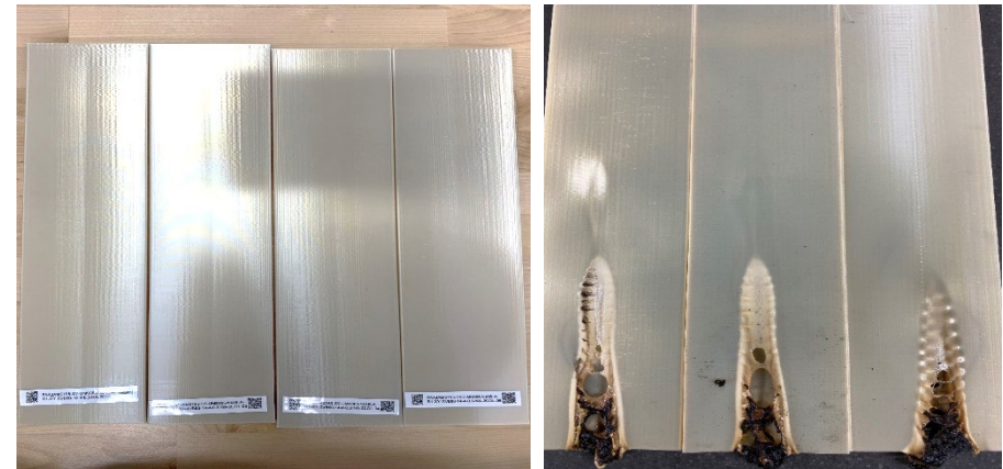
Pre (left) and post-test (right) vertical burn test specimens
