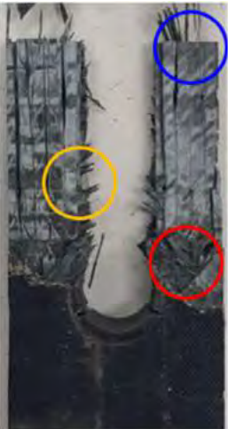
Hexcel Carbon/epoxy Open-hole Sample [\pm 45/0_2/90/0_2/\mp 45]_9
