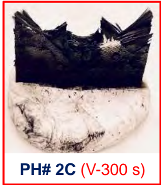
PH# 2C (V-300 s) Typical Fracture Morphologies Observed after Nitric Acid Oxidation
