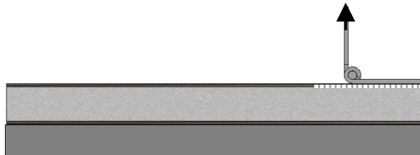
Plate-Supported Single Cantilever Beam
