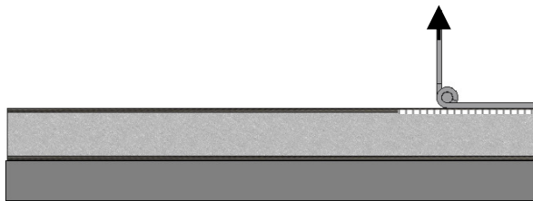
Plate-Supported Single Cantilever Beam (SCB)
