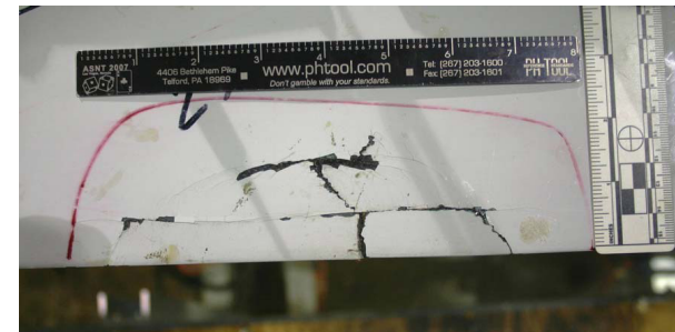
Damage on Aft Leading Edge
