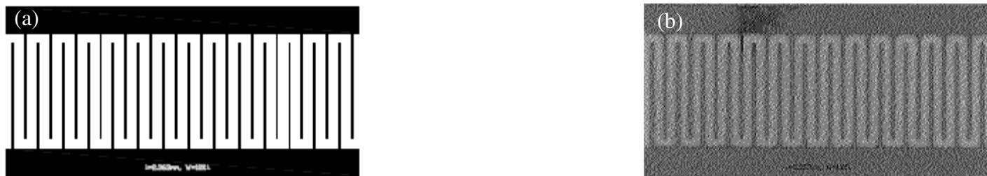
Fig. 6: (a) Electrode pattern design for the interdigital transducer with finger spacing of \Lambda=2.363 mm and finger width of 20% \Lambda ; (b) Electrode pattern on a PZT transducer fabricated with photolithography (Dark areas: Nickel electrodes).
