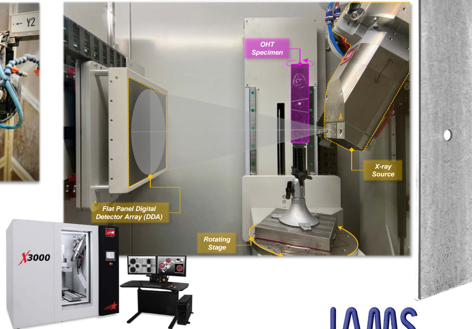
X-Ray Computed Tomography Inspection
