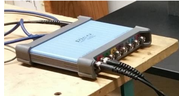
Easily portable Picoscope 4824 oscilloscope
