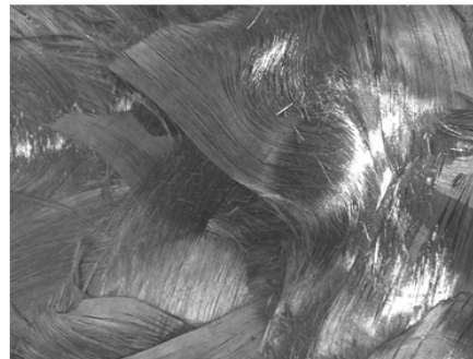
Large chip aligned distribution Some curved fibers Some intertwining of layers
