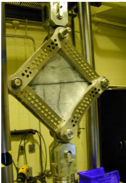
Picture Frame Shear Test Set-Up
