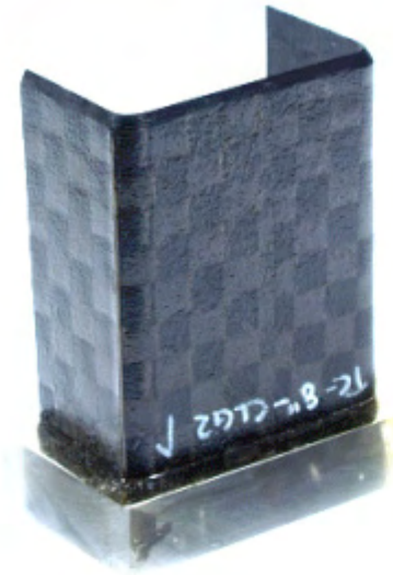
Figure 8 a, b. Large C-channel, specimen II, before and after crush testing.
