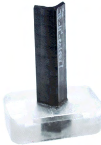
Figure 10 a, b. Small corner element, specimen IV, before and after crush testing.
