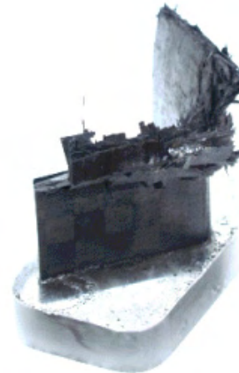
Figure 10 a, b. Small corner element, specimen IV, before and after crush testing.
