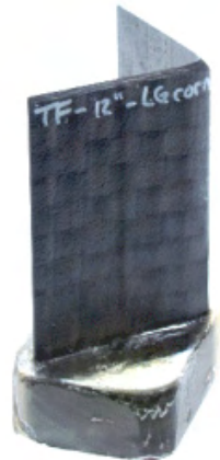
Figure 10 a, b. Small corner element, specimen IV, before and after crush testing.
