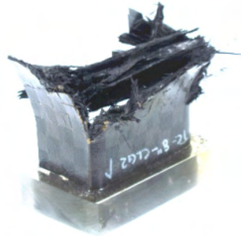
Figure 8 a, b. Large C-channel, specimen II, before and after crush testing.
