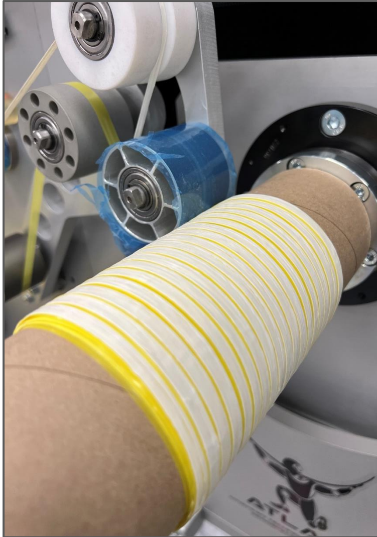
Proper resin/tack level
