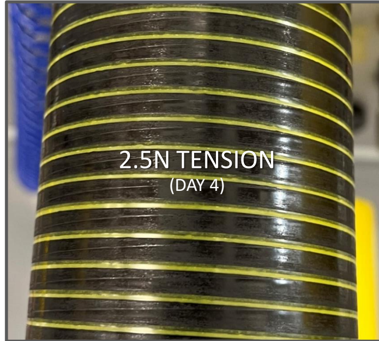
Poly tension optimal and aligned with material
