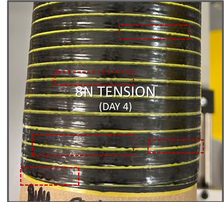
Higher poly tension caused material bubbling
