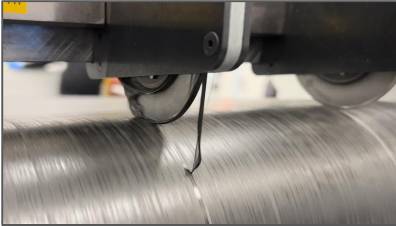
Removing poly pre-cut results in fiber pull
