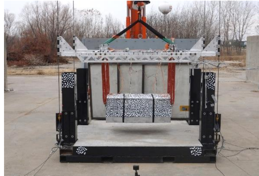
Pre-Test Image: Mounted Battery Pack
