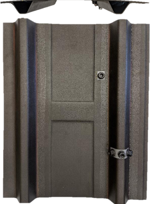
2-Stringer panel with added mass (2cm diameter steel nuts) simulating damage
