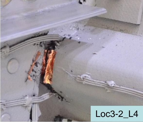
Stringer cut by shear tie
