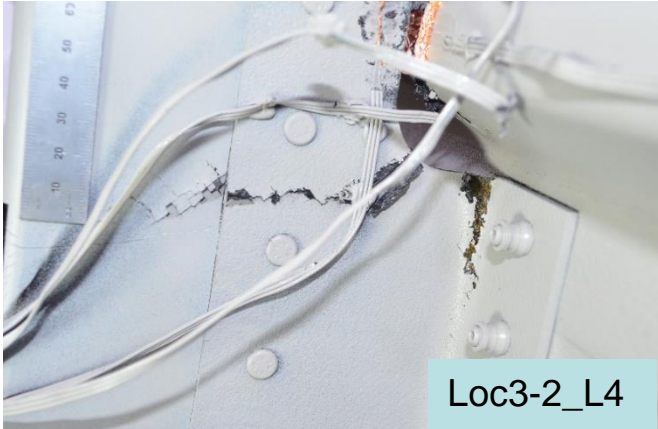
Shear tie crack originating from mouse hole and following C-frame crack
