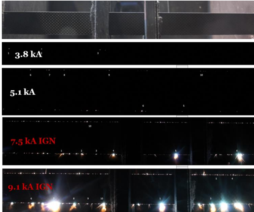
Testing in flammable gas mixture (6 vol% hydrogen and dry air)
