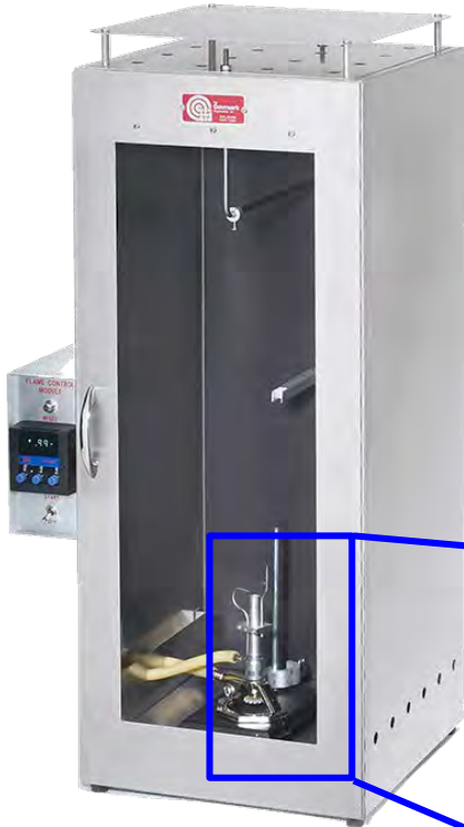
Draft-free Vertical Bunsen Burner Test Cabinet [4]
