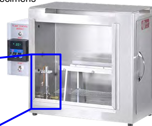
Draft-free Horizontal Bunsen Burner Test Cabinet [4]
