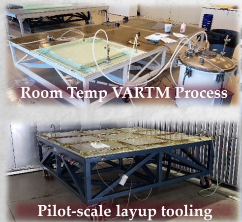
Temp & Humidity Controlled Layup
