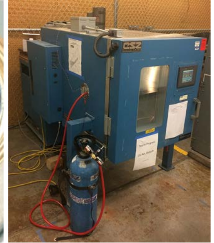
Exposed Amine Component (Left) Environmental Conditioning Chamber (Right)
