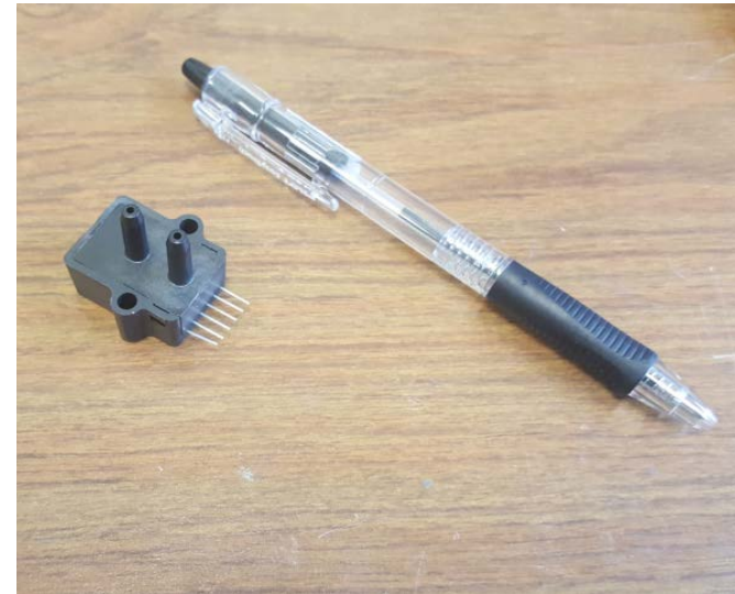
All Sensors Type MLV-015A-A6-AAF-N pressure sensor with 0-15 psi pressure range (absolute)
