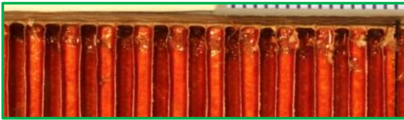
Core crushing span for 590 J energy: ~76 mm
