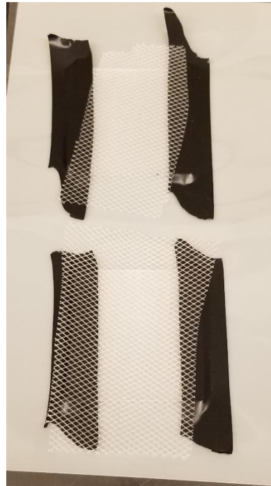
VARTM mesh removal
