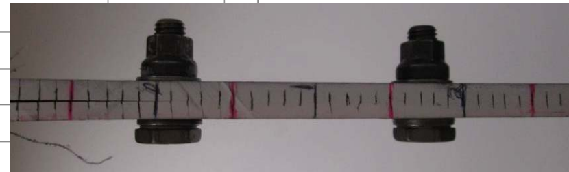
Test Sample with crack forced into Mode II
