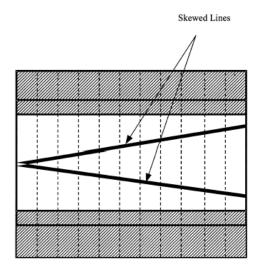
Figure 1 – Specimen Traceability Line
