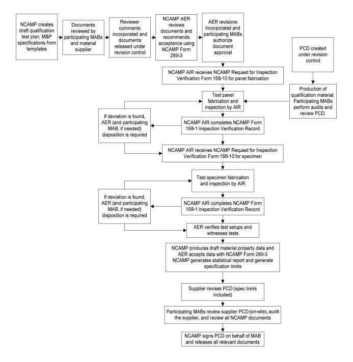
Figure 2. Flowchart of Material Qualification and Property Data Acquisition Process
