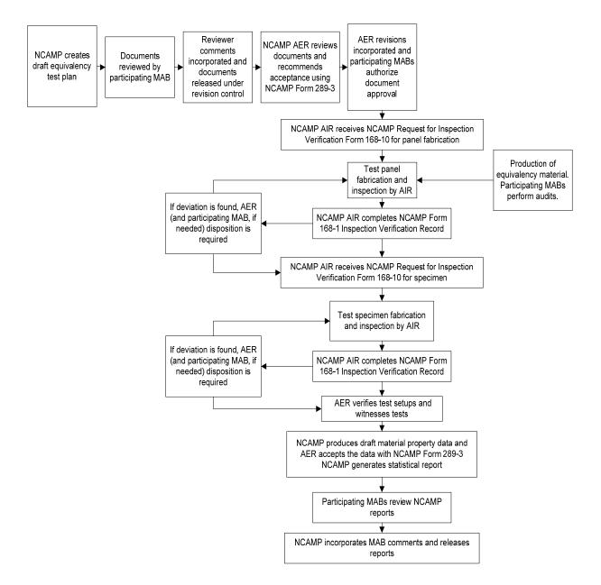
Figure 3. Flowchart of Equivalency Process for Part Fabricators
