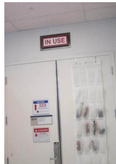
Figure 1: Laser Warning Sign Too High and Not Informative
