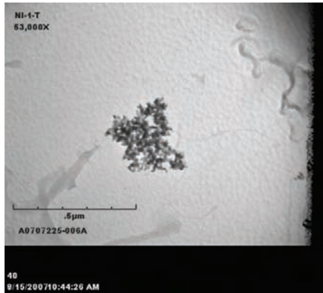
Figure 5. Electron microscopy micrograph of an agglomerated nanoparticle of nickel oxide
