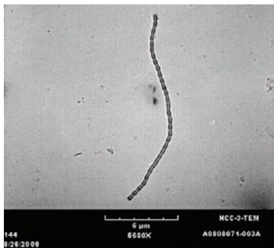
Figure 3. Electron microscopy micrograph of a carbon nanofiber
